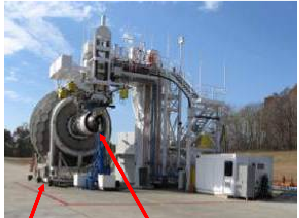
Inlet Turbulent Control Structure
