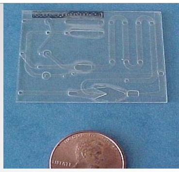
Under development with Micronics and Honeywell for DARPA is a complete cytometer to fit in a wristwatch.
