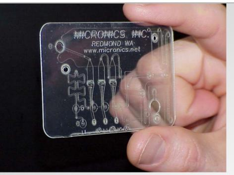
Micronics demonstrates complete fluidics for a flow cytometry system on a 7-layer microfluidic card
