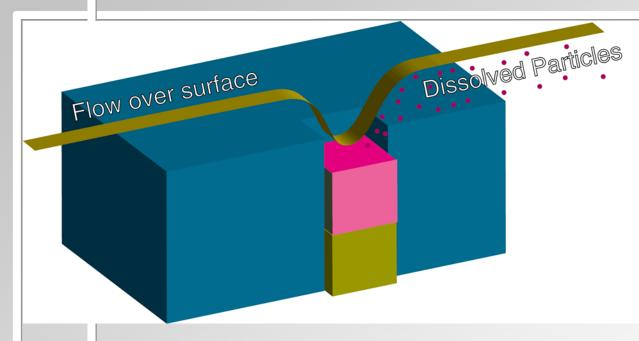
How to create controlled streams of multiple reagents without multiple pumps? Blocks of one or more materials dissolve as the fluid flows over them.
