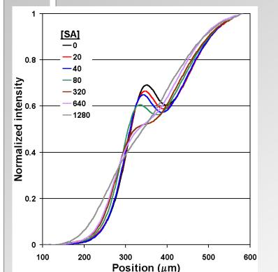
Modeling: a 1D simulation of the phenytoin experiment
