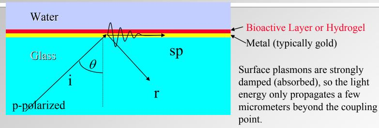
For a given metal film thickness, light at one frequency will, at a particular angle  $\theta$ , resonate with plasmons in the metal film.
