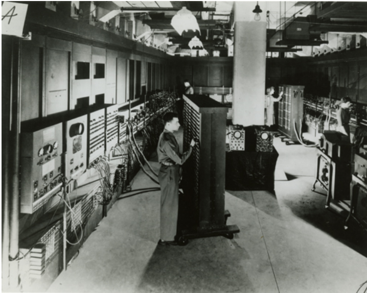
ENIAC (constructed 1943-1946) [8.5' (h) x 3' (d) x 80' (linear), 30 tons, 17,468 vacuum tubes, 150 kW of power, 5,000 additions/second]
