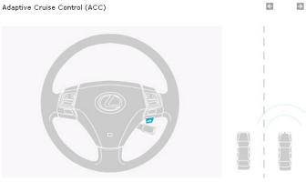
If traditional cruise control had a higher IQ, this would be the result. Adaptive Cruise Control (ACC) works just like a more conventional cruise control system - until it detects a car in front of it. Sensors detect that you are approaching a car ahead.
