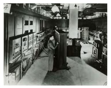
ENIAC (constructed 1943-1946) [8.5' (h) × 3' (d) × 80' (linear), 30 tons, 17,468 vacuum tubes, 150 kW of power, 5,000 additions/second]
