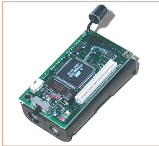
Figure 1. Mica wireless sensor platform. The node measures 1.25 x 2.25 inches, as dictated by the two-AA battery power supply, which supports applications that last for several years. Mica was developed as a low-cost, energy-efficient, experimental platform, and a single-chip version of the architecture is in development.
