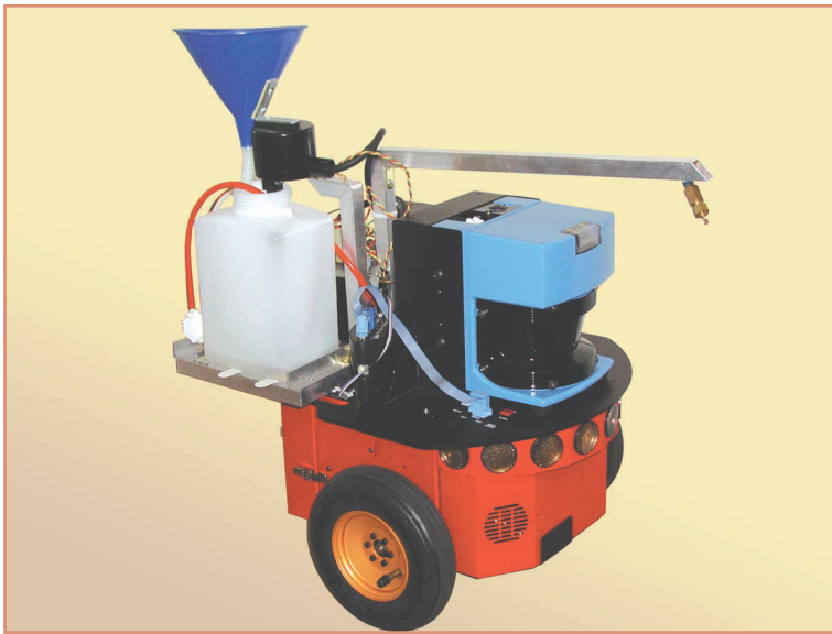
Figure 2. The Plant-Care robot hardware platform consists of a Pioneer 2-DX mobile robot with custom hardware for watering plants, inductive charge coils for recharging both the robot and the deployed sensors, a laser scanner used for navigation, and an IEEE 802.11-enabled laptop that runs the robot's control and navigation software.
